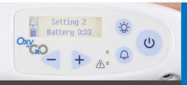
OxyGo shows you how much time is left before you need to recharge or switch batteries
